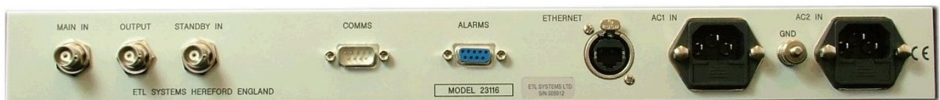
Rear View of Model 23116-B5B5 (with 50 ohm BNC connectors)
